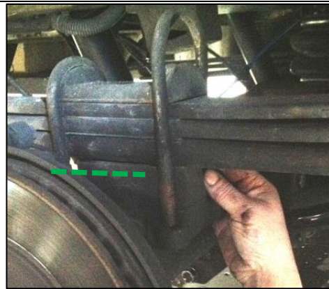
Removal of U bolts
