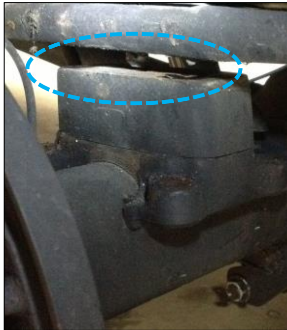
Original position of extended leaf spring spacer
